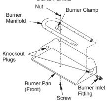
Figure 6 - Installing Burner
